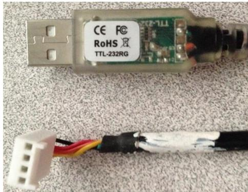
Figure 1: Serial-To-USB Adapter cable
