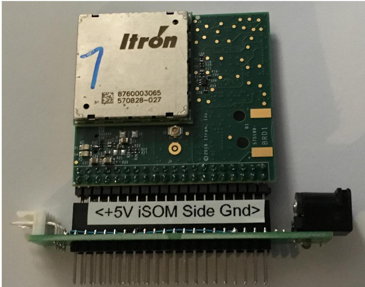
Figure 6 - ACT NIC on Solderless Breadboard Expansion Board
